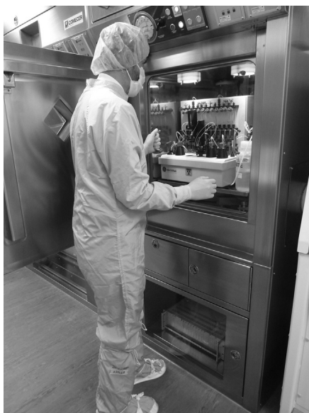
Figure 45.5 • Synthesis module for ^{18}\text{F} -FDG production (TRACERlabF x Synthesizer®). (Courtesy of GE Healthcare plc.) Module located in lead-shielded (5.5 cm) specialized fume cupboard known as 'hot cell'.
